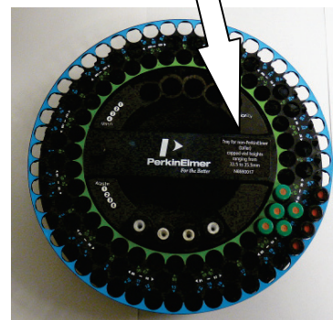
108-Vial Tall Tray and Carousel (for non-PerkinElmer vials)
