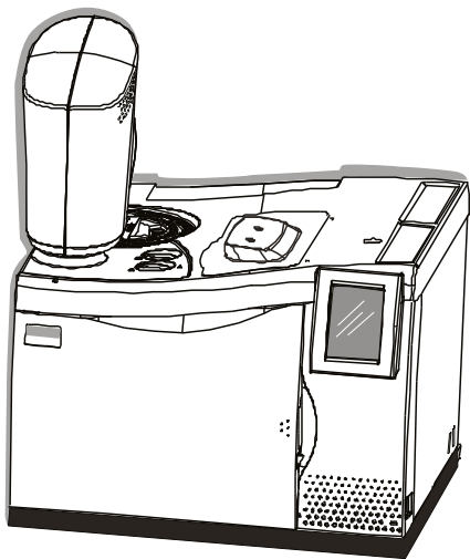
Figure 3-9. View of the Clarus GC with autosampler tower.
