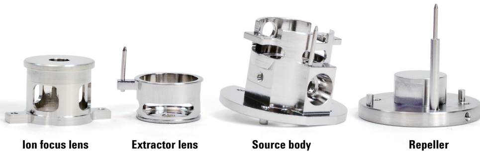
Figure 27 Extractor EI Source parts to be cleaned
